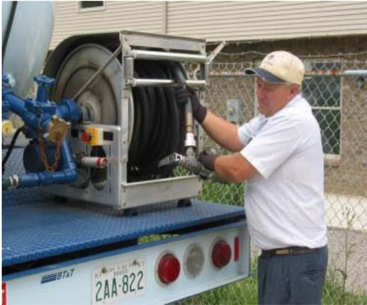
U.S. DOT cargo tank unloading regulations require specific delivery hose and emergency discharge system inspections during each unloading operation. Additional monthly and annual inspections of delivery hoses and testing of the internal self-closing stop valve ("belly valve") are required as well. This applies to all operators of cargo tank motor vehicles.
