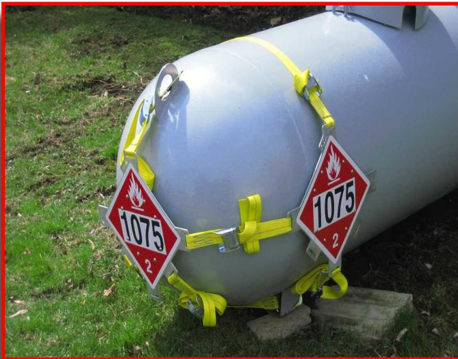
When transporting a portable propane tank up to 999 gallons water capacity, it must be legibly marked on two opposing sides with the proper
